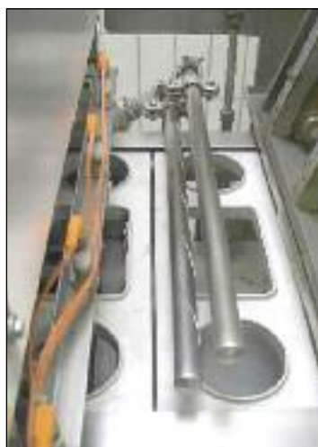
Integration of an active air degermination unit in a filling machine (left) and a ventilation duct (right)
