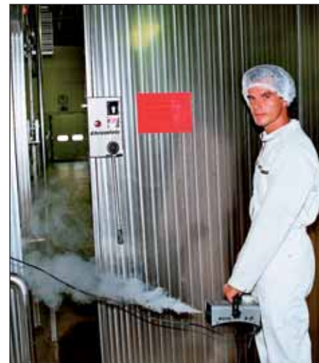
Robert Kuhl visualizes the air flow with a fogging unit
