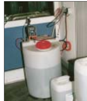
20 L cans are used for refilling the 100 L storage container needed for machine degermination.
